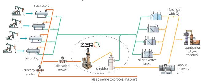
Figure A8 Typical application of the EcoVapor ZerO<sub>2</sub> technology<sup>41</sup>
